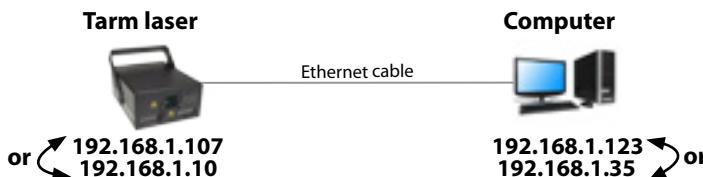
Laser devices as tarm four and tarm seven have their own default IP address 192.168.1.107. In order to establish the connection, connect the laser device through the ethernet cable directly with the laptop or PC.
